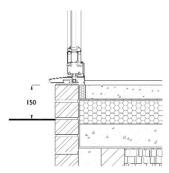
☐ Level with gap between extended cill and flags for drainage
