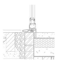
☐ Flush with stainless drain abutting doors
